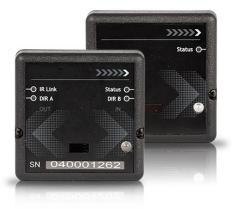
Operation principle: infrared beam crossing Movement direction finding: two directions IN and OUT Internal memory: 1000 records Measurement period: 5-min in graphic reports, 1-sec in raw data format Battery life: up to 1 year Communication range: up to 800m Additional feature: real-time data delivery to a server
